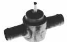
26-0296 Heater control valve 5/8" brass. Bottom threaded Fe 8-32 x 10 (2x)
