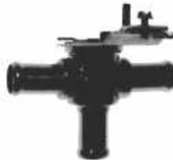
26-0043 Heater control valve 5/8" 3-way. Inlet from bottom when bracket on top*. Pull for waterflow to left side.
