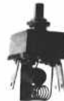
25-0028 For 3 speed motors, 15 amp with resistor, 4 pos. Must be mounted in the air stream for cooling
